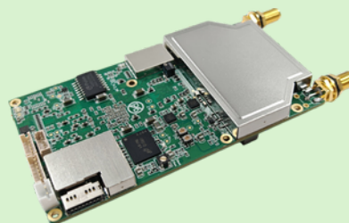
11.5×5.4×1.3cm/56g 4Watts×2/5Watts×2 (Air to G. 100~150/100~200KM)
