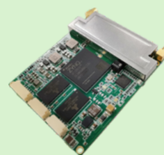
5.8×4.8×1.0cm/27g 0.5Watts×2/1Watts×2 (Air to G. 10~30/20~50KM)
