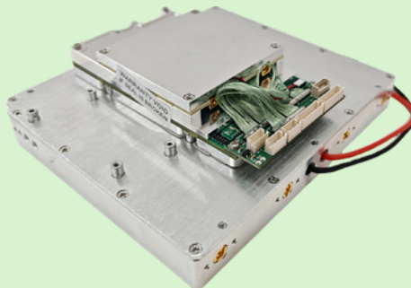
12.7×11.0×3.6cm/575g 10Watts×2/20Watts×2 (7Z030/7Z035) (Air to G. 150~300/250~500KM)
