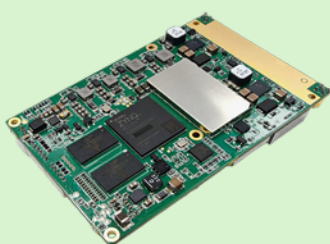
8.7×5.4×1.0cm/43g 1Watts×2/2Watts×2 (Air to G. 20~50/50~100KM)
